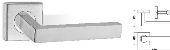
AMH-11 Mortise handle solid casted Finish : Satin / Glossy Material : Stainless steel 304 grade (Also available in plate type mortise)
