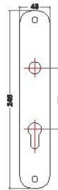
AMH-02-P Mortise handle with plate Finish : Satin / Glossy Material : Stainless steel 304 grade
